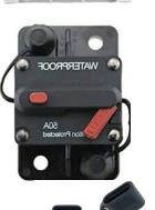
Circuit breakers must be fitted to onboard battery chargers. The circuit breaker rating must be slightly higher than the max DC output of the charger. Batteries must be isolated when charging and battery chargers must be isolated when in storage. LED lights and screens i.e standby power flattens and unbalance lithium batteries. Fuses are recommended to be installed to protect against incorrect connection.
