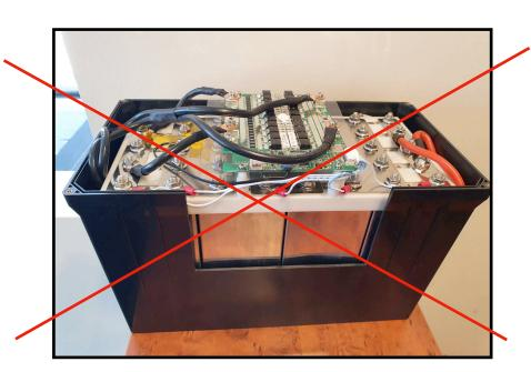
12V 20P 4S = 40 cells 4 BMS wires
