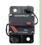
Circuit Breakers are required to protect cables and appliances such as trolling motors. Fuses protect appliances. The circuit breaker rating must be slightly higher than the total amp/current draw on the circuit. Circuit breakers can be used to isolate circuits and chargers from lithium batteries
